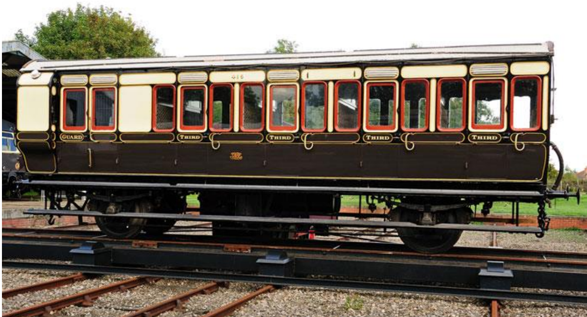
The only remaining example of a Dean 4-brake third class coach as used by GWR in late 19 th C. The guard's compartment can be seen on the left. Photograph courtesy of Didcot Railway Centre and Frank Dumbleton.
