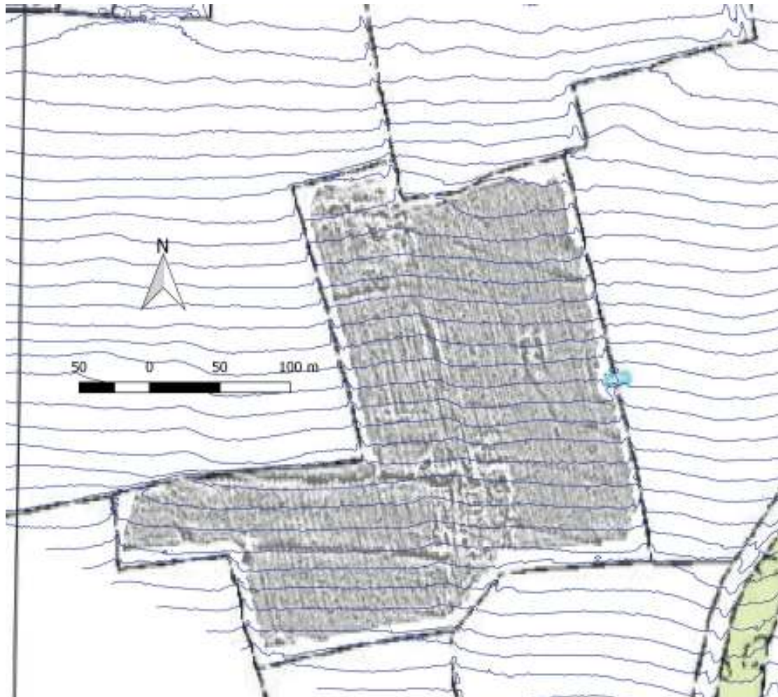
Figure 3.9. Magnetometry overlaid by 1 m contour map to provide extra detail. Note steeper bank towards southern end of field – contours are closer for 1 m. Heights have not been included to avoid extra clutter. For absolute heights, refer to figure 3.8.
