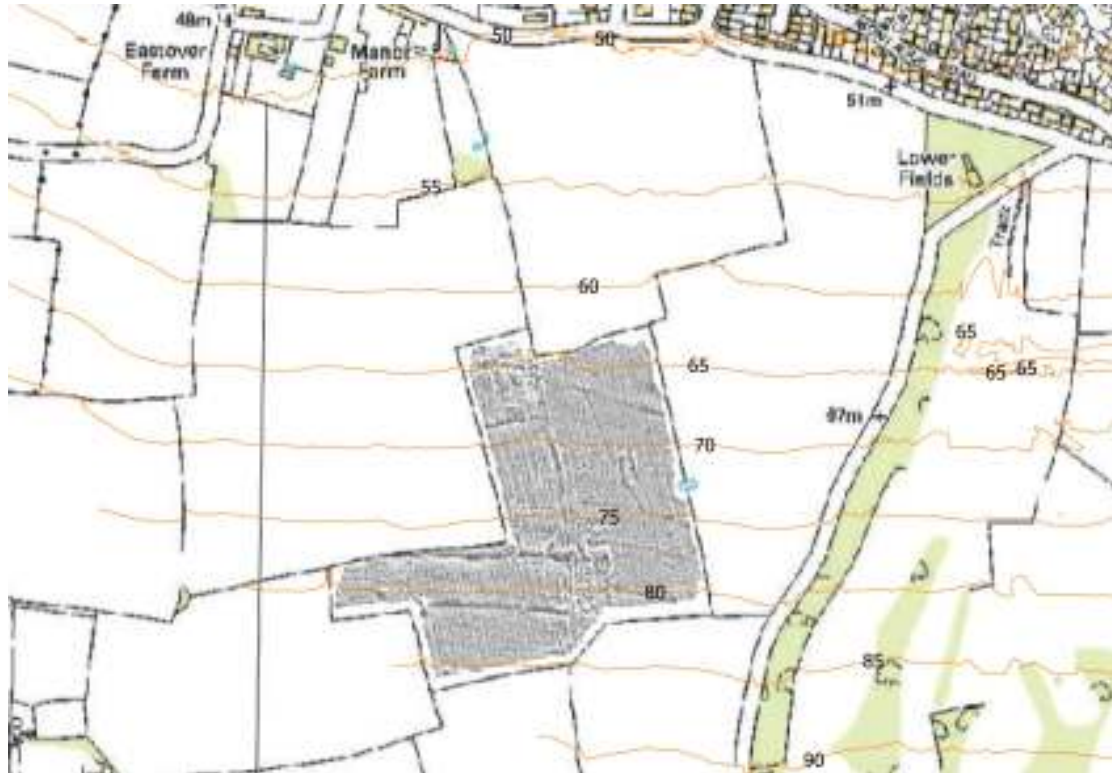
Figure 3.8. Lidar-generated contour map (5 m interval), showing Coffin Field geophysical survey and surrounding fields. North to top. The irregular areas of contour on the right show earth movements on the nearby golf course.
